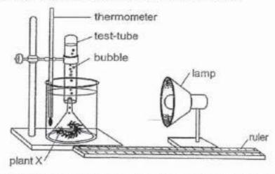
She switched on the lamp and counted the number of bubbles produced by plant X in one minute.
