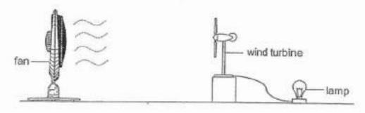
Meiling placed the wind turbine closer to the fan. She observed that the blades of the wind turbine spun faster and the lamp lit up more brightly.
