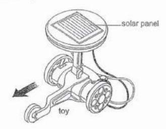
When the toy is placed under the Sun, the solar cell in the solar panel absorbs energy from the Sun and the toy moves forward.
