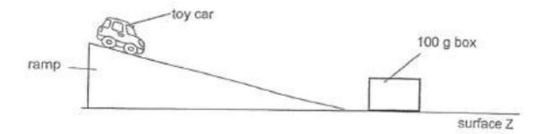
He released the toy car from the top of the ramp and recorded the distance travelled by the 100 g box on surface Z. He repeated the experiment with a 400 g box of the same size.
